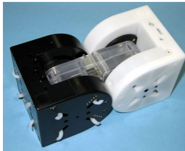
Figure 2.1: MTRAN III module. Picture is taken from [5].
