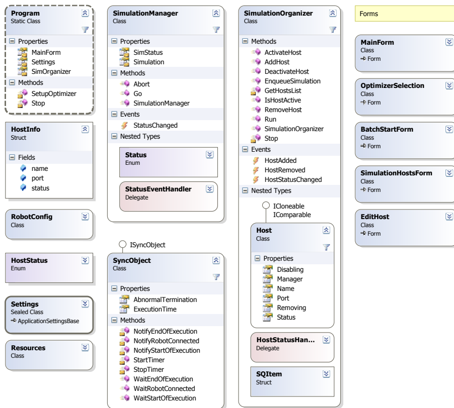
Figure 5.14: YaMoR Optimizer class diagram
