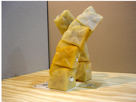
Figure 2.3: Molecube (8 modules here). Picture is taken from [7].
