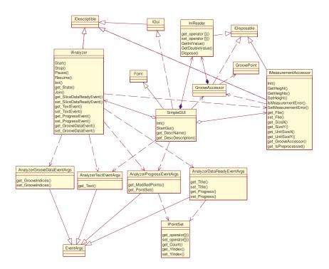
Figure B.5: Class diagram for SimpleUI
