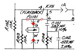
Figure 5.2: Schematic of playback needle connection.
