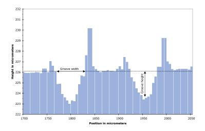
Figure 3.3: Cross-section of measured surface showing two grooves.
