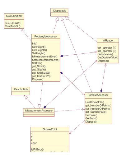
Figure B.4: Class diagram for Rectangle Accessor
