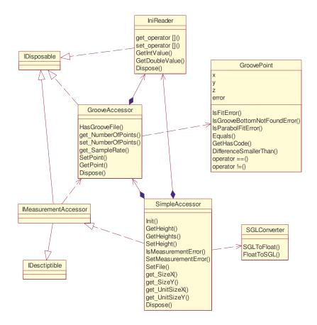
Figure B.3: Class diagram for Simple Accessor
