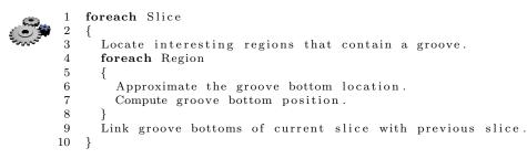
Different approaches were investigated to compute the best possible groove bottom position. All of them fit a certain function, which is a model of the stylus geometry, to the neighbor data points of the first approximation. The next subsections describe these different techniques.
