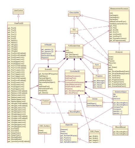
Figure B.9: Class diagram for Full3D
