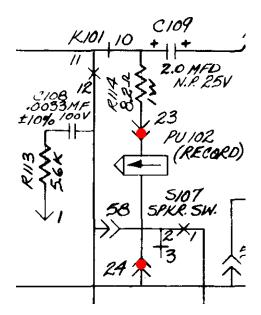
Figure 5.4: Schematic of the recording needle connection.
