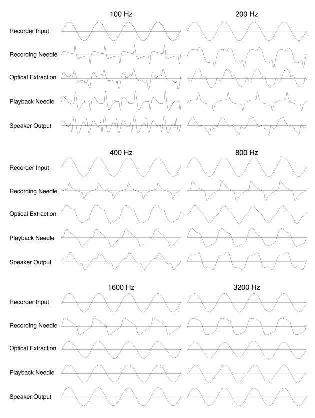
Figure 7.1: Signal applitude comparison.
