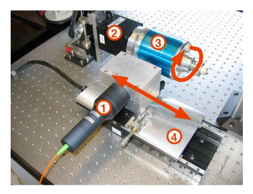
Figure 3.5: Overall setup of the measurement hardware. 1. is the confocal probe, 2. is the rotational stage and encoder, 3. is the dictation belt mounted onto a aluminum cylinder and 4. is the linear stage and encoder. The red arrows show the motion of the rotational and linear stage.
