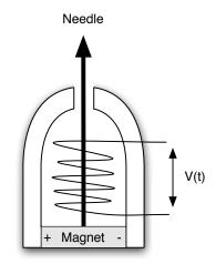
Figure 5.3: Schema of the recording needle.
